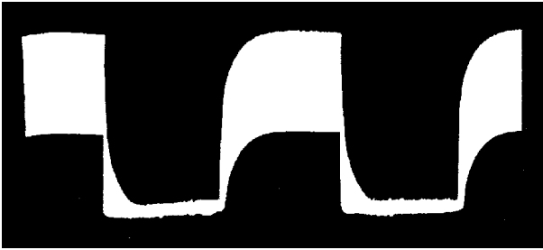
21-4 PIN diode switching using square-wave chopper waveform.
