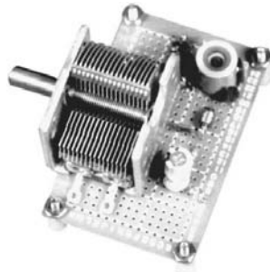
1-7 VFO circuit build on perftboard.
